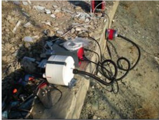
(a) Shaker system (shaker, cooling and power amplifier)
