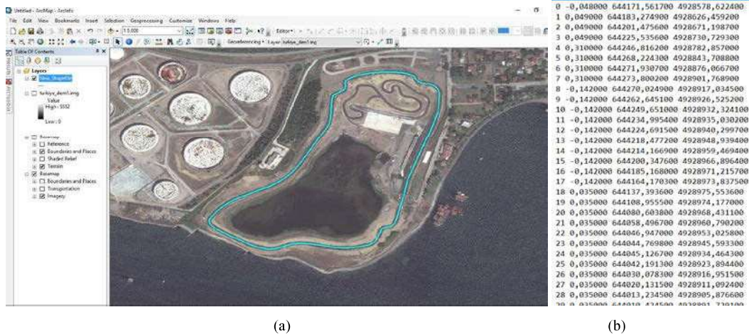
Fig.5. (a) Processing the coordinates and slope values of the route in different layers with ArcGIS software environment from Geographical information systems, (b) Transferring processed data to a text file.
