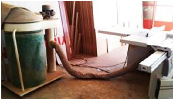
Fig. 3. Collection of dust generated during the cutting of wood by suction using a vacuum system.
