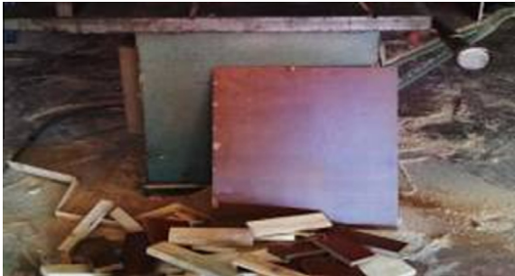
Fig. 4. Small pieces of board left over after the cutting of larger boards.
