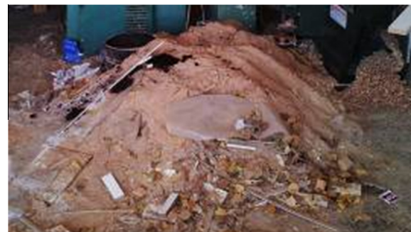
Fig. 2. Wastes generated during the processing of MDF and particleboard in furniture manufacturing.
