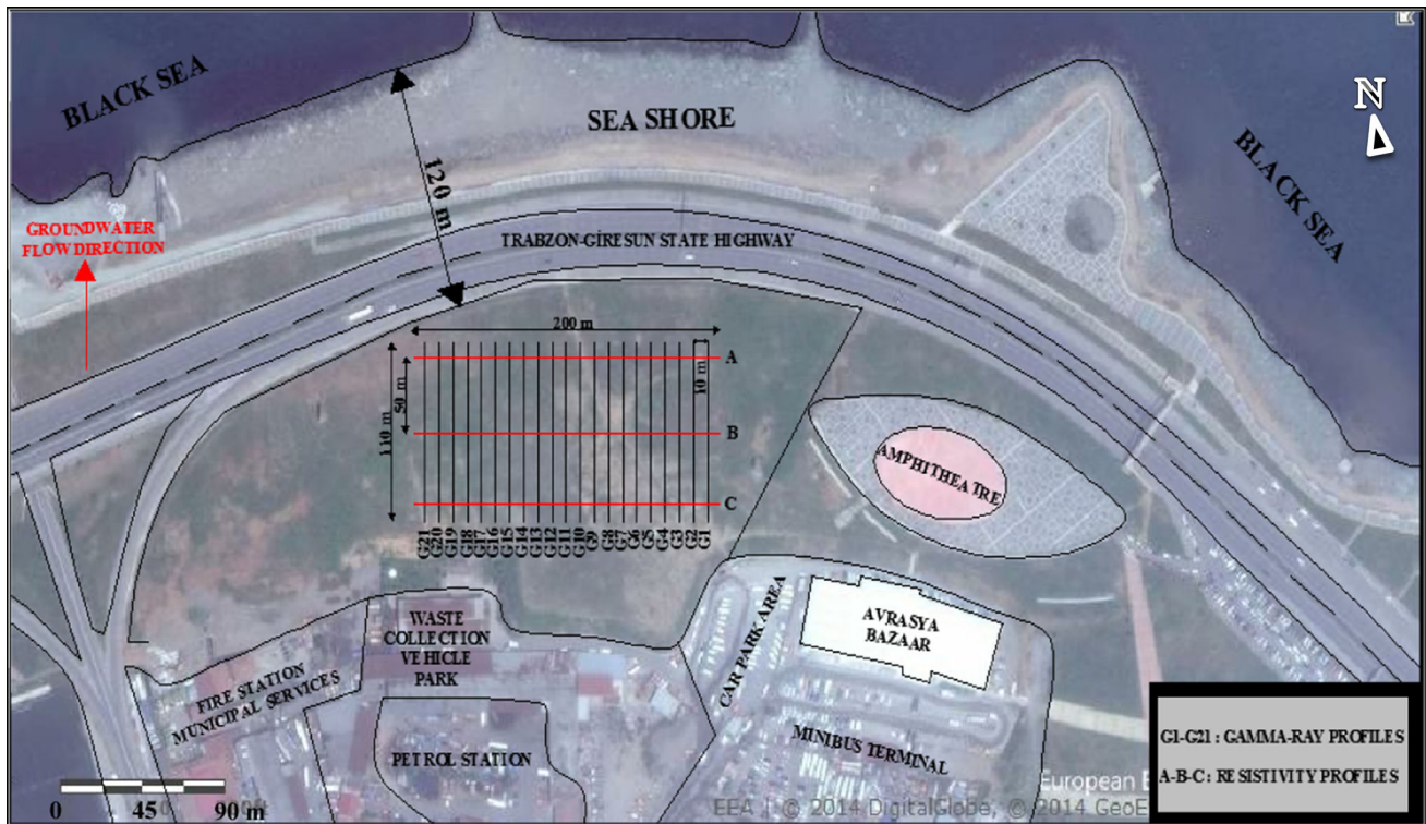
Fig. 2 A schematic sketch showing studied area (resistivity profiles are “red lines” and gamma-ray profiles are “black lines”). Actual data point locations are shown Fig. 6 (modified from Google Earth 2013)
