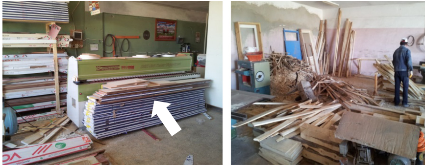
Fig. 2. Examples of inappropriate storage of partially finished products and materials.
