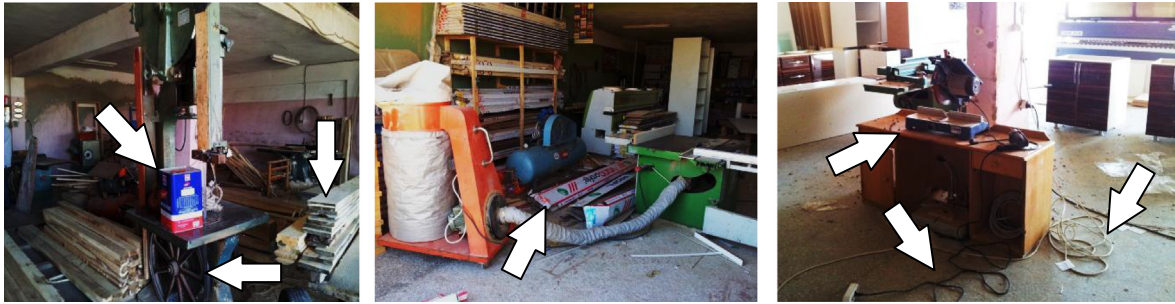
Fig. 1. Examples of poor practices that may lead to accidents: (left) unguarded moving parts, (centre) obstructed working space and (right) exposed cables.
