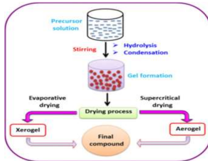
Figure 1. The stages of the sol-gel formation process.
