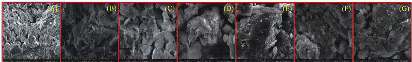
Fig.5. The SEM images of the pristine montmorillonite and surfactant modified montmorillonite samples A) MMT B) C_{16} TABr/MMT C) C_{14} TABr/MMT D) ( C_{16} )ABr/MMT E) C_{12} TABr/MMT F) C_{10} TABr/MMT G) C_8 TABr/MMT
