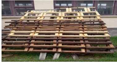
Fig. 1: Inclined platform of test samples stored in the external environment.
