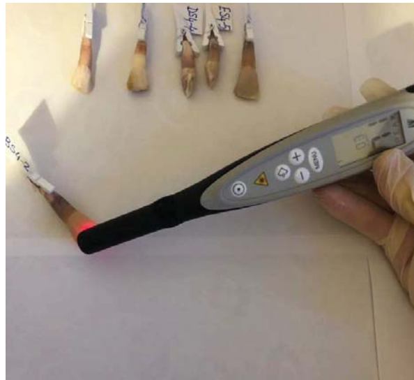
FIGURE 1. Baseline measurements for the teeth to be included in the study with DD.
