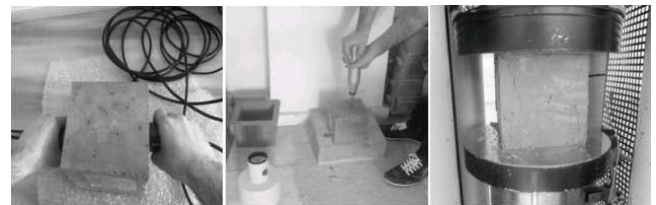
Fig. 1. Ultrasonic pulse velocity, Schmidt hammer and compressive strength test methods.
